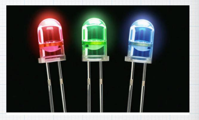
Using an LED is very simple, but there are a couple of precautions. First, you must *always* have a resistor in series with it. Without the resistor, you run the risk of having the diode current become too high, causing the diode to burn out. The value of the resistor is not critical anything between 100  $\Omega$  and 1 k $\Omega$  is probably OK, although lower resistance values will give a brighter output.
