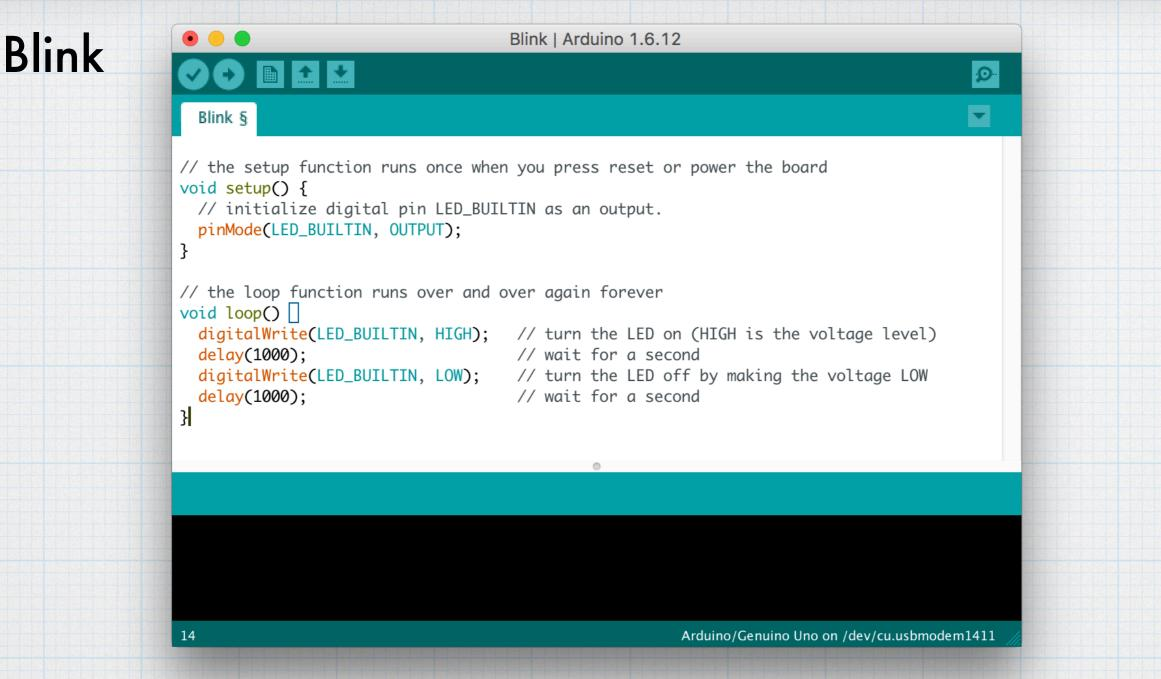
At the end of the previous lecture slides, we loaded and ran the blink program. When the program is running, the built-in LED blinks on and off — on for one second and off for one second. It is very simple, but it consists of functions that are not familiar: pinMode, digitalWrite and delay. However, it is not hard to guess the purpose of these functions. We will look at them in more detail.
