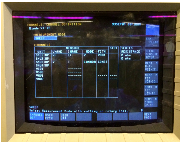
Figure 4. Channel definition page with the SMUs set up for a diode measurement.
