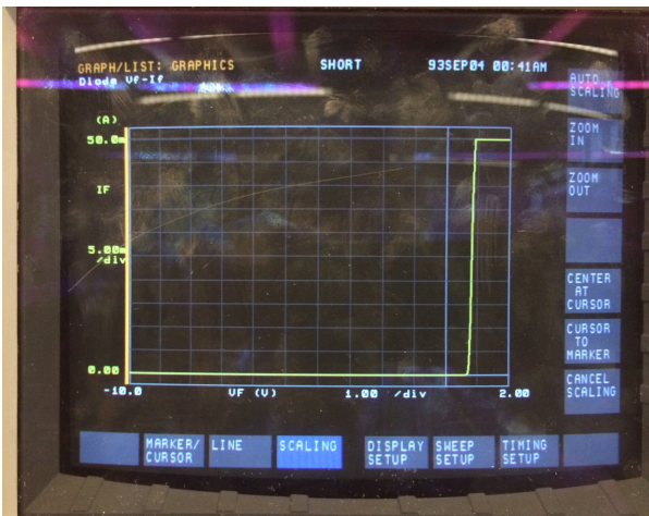
Figure 8. Diode curve after auto-scaling. It is classic. Note that the forward characteristic flattens off at 50 mA. This is due to the current compliance limit that was set on the Sweep Setup page.
