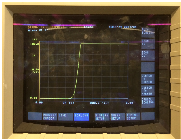
Figure 10. Forward characteristic of the diode on linear scales. Once again, note how the compliance limit has flattened the top of the measurement.
